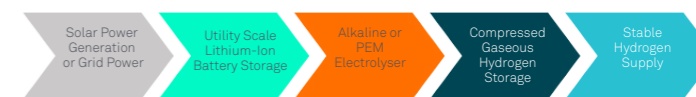
Figure 1 Modelled steps of the hydrogen value chain (with or without grid connection).
